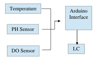
Network (WSN) that helps to monitor the quality of water with the help of information sensed by the sensors immersed in water. The parameters such as pH,amount of dissolved oxygen, temperature, etc. Are been monitored.
